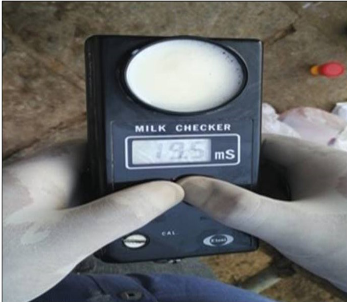
Figure 4: Detection of mastitis by EC test using milk checker instrument
